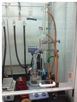
A Dean–Stark apparatus in use; aluminium foil is used to reduce heat losses
